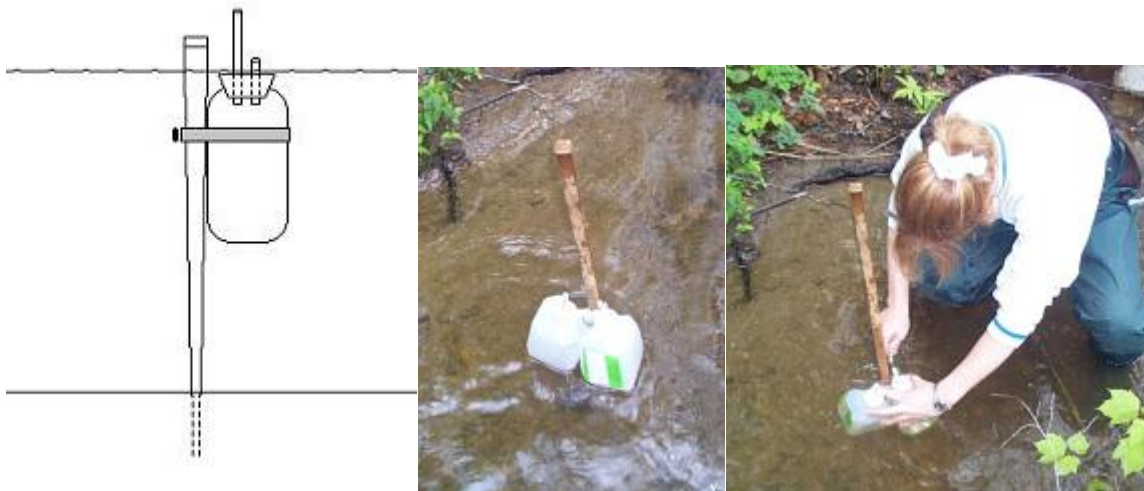
Figure 30. Passive storm water sampler for collection of first flush storm water.
